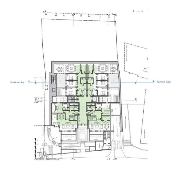
Plan of proposed building with a typlical floor of the existing building overlaid (in Green) one of the 3 proposed basments levels.
