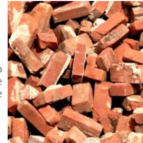
Old Bricks to Concrete Aggregate
