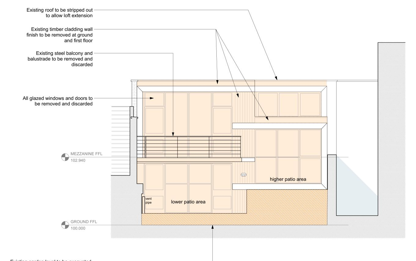
Existing garden level to be excavated. — Exterior floor level to be lowered to match interior existing ground floor FFL
