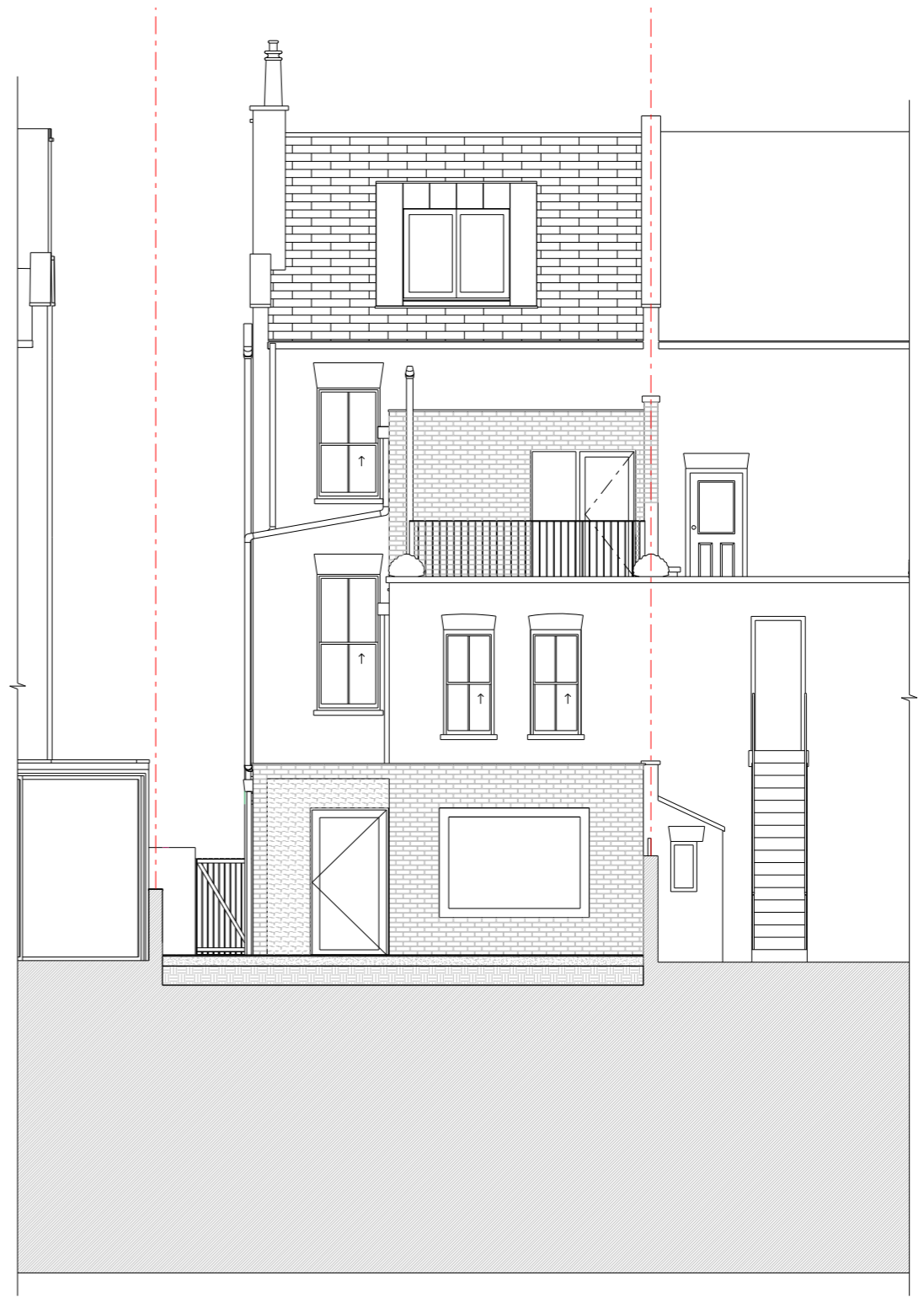
02 EXISTING NORTH ELEVATION 1:100 @A3
