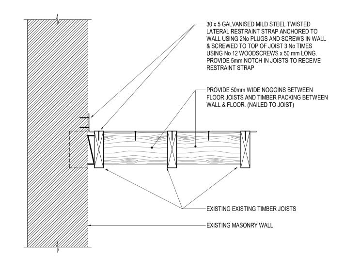
RESTRAINT TO EXISTING WALL PERPENDICULAR TO JOISTS
