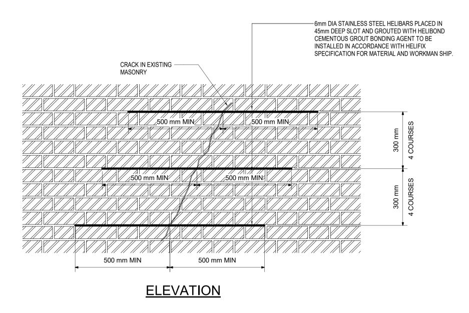
DIAGONAL CRACK REPAIR DETAIL (TYPICAL)
