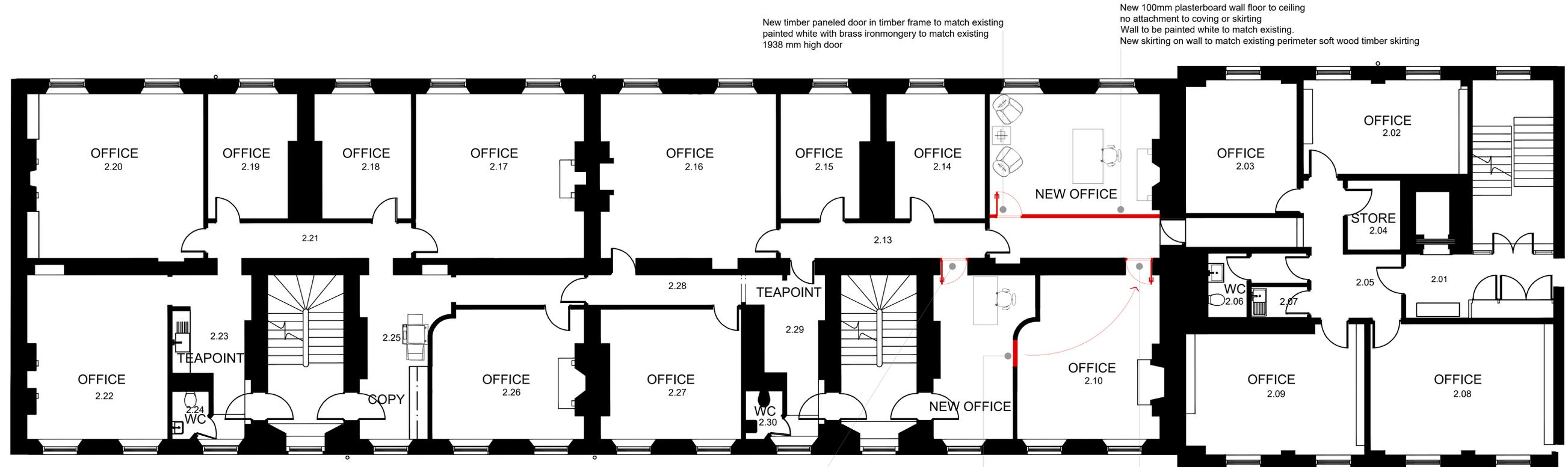
New timber paneled door in timber frame to match existing painted white with brass ironmongery to match existing 1938 mm high door
