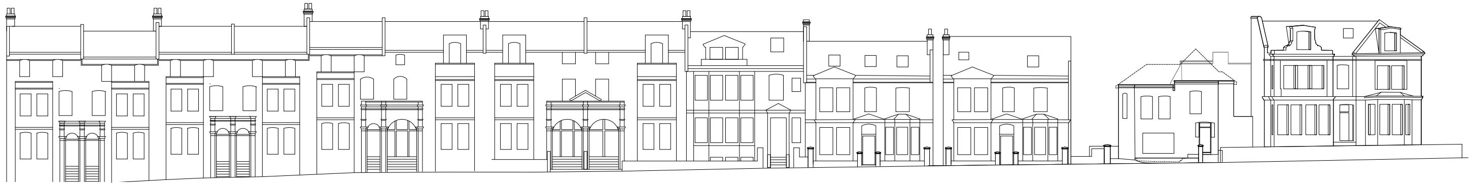
Elevation of Hilltop Road. The approved roof extension scheme is shown with dashed line.
