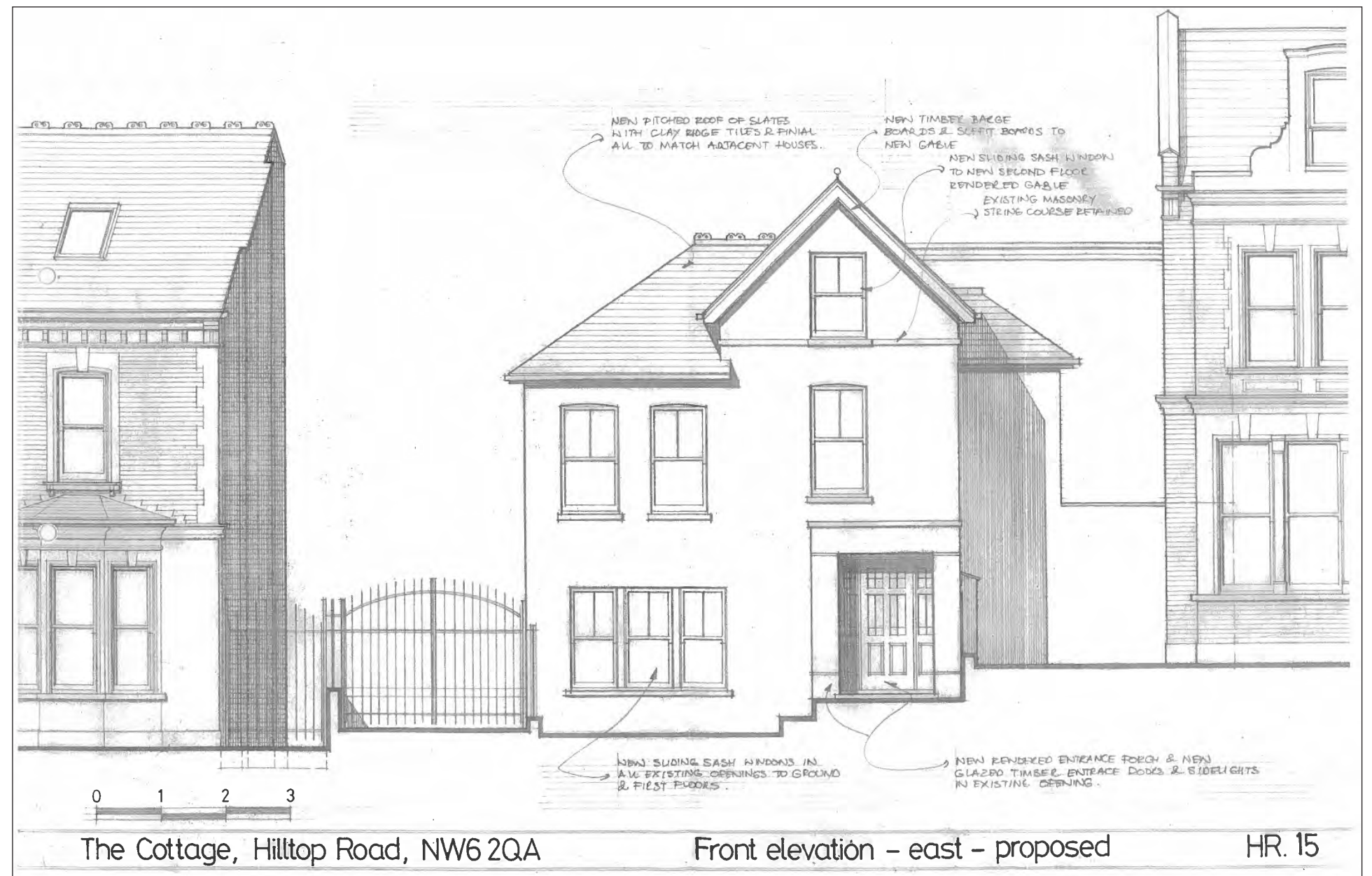
Proposed front elevation for the roof extension.
