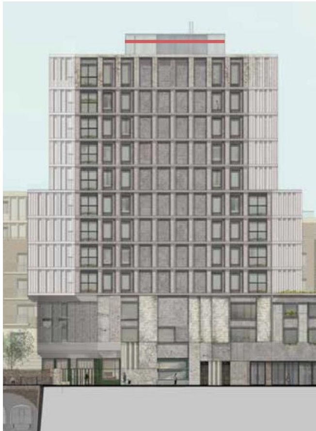
Figure 4.2: Section through residential building indicating increased lift overrun and new flues (above the red line) (Source: AHMM)
