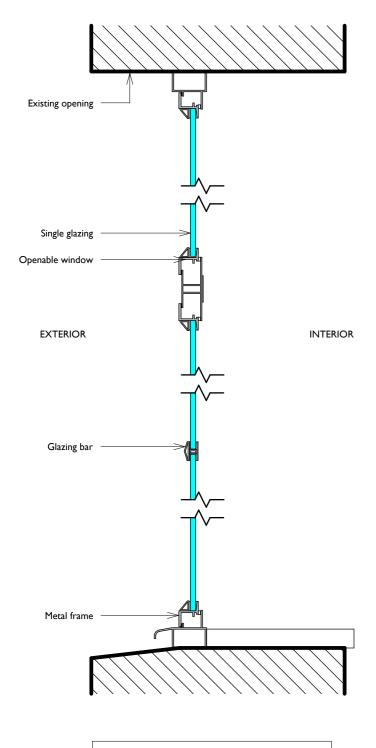
Section of window is assumed based on photographs of existing condition.
