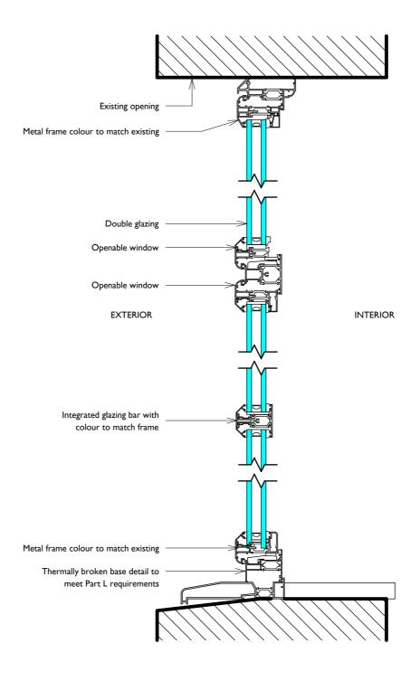
Section of window based on thermally broken Alitherm 300 system.
