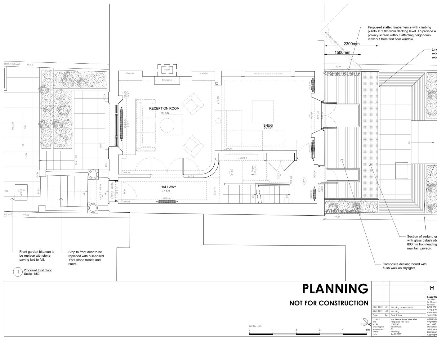
privacy screen without affecting neighbours view out from first floor window. Line of proposed rear extension 2.3m from existing rear facade. ead  $\wedge$ N. 10 Section of sedum/ green roof with glass balustrade set back 800mm from leading edge to maintain privacy. Composite decking board with flush walk on skylights.
