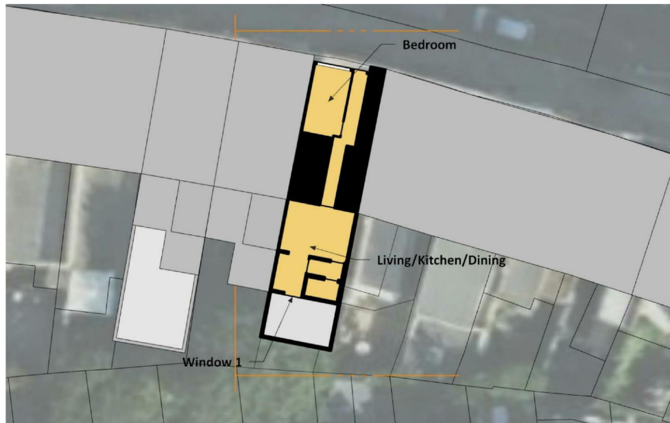
Fig 8. Section cut through ground floor showing proposed layout with habitable rooms and windows tested for sunlight hours labelled. North to top.
