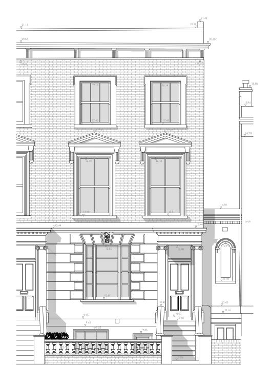
Proposed Front Elevation Scale: 1:75
