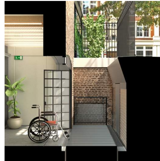
Fig. 6. Lightwell platform lift at its default position on the lower ground level
