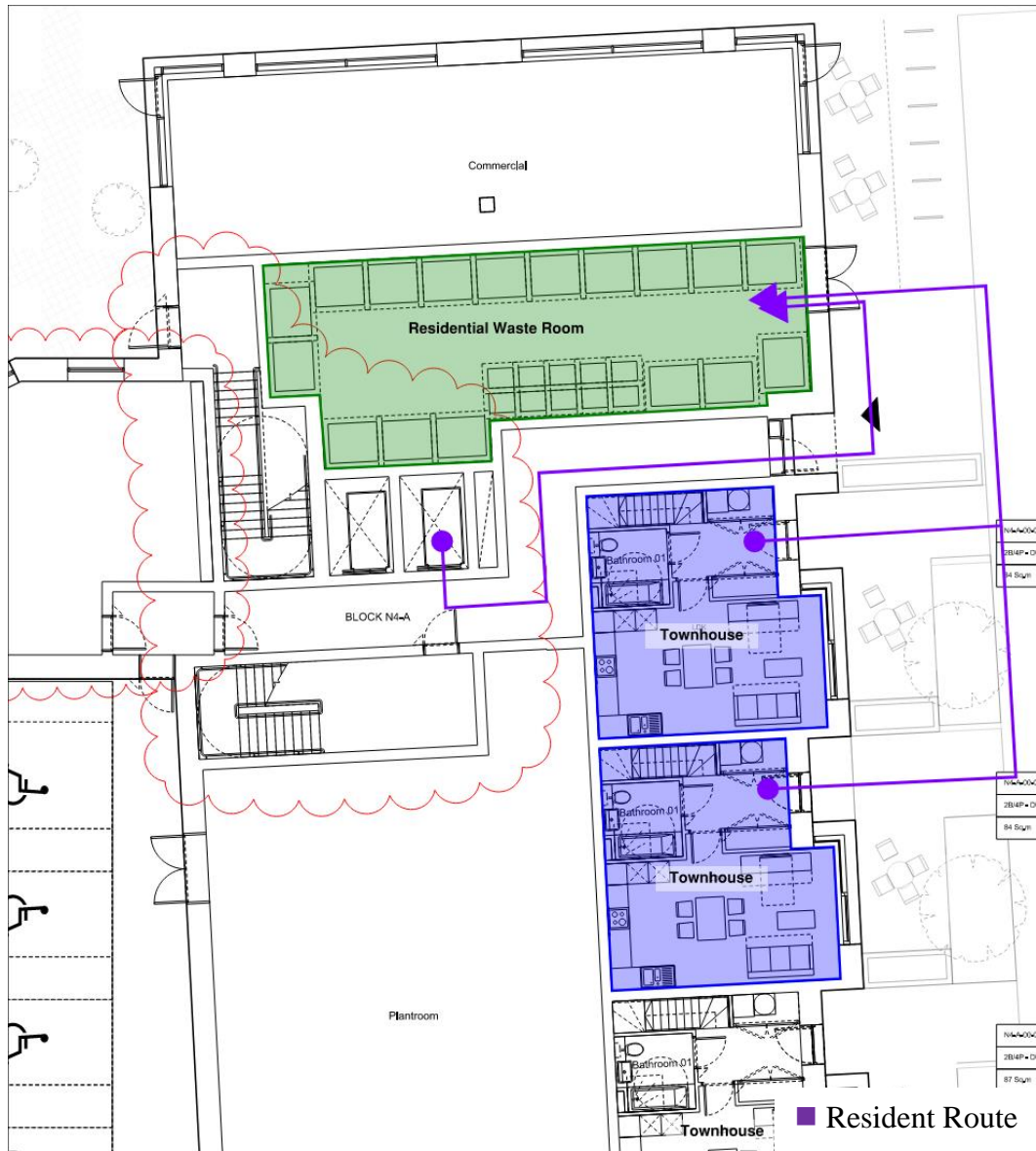
Figure 4: Residential waste conveyance route N4-A (ground floor)
