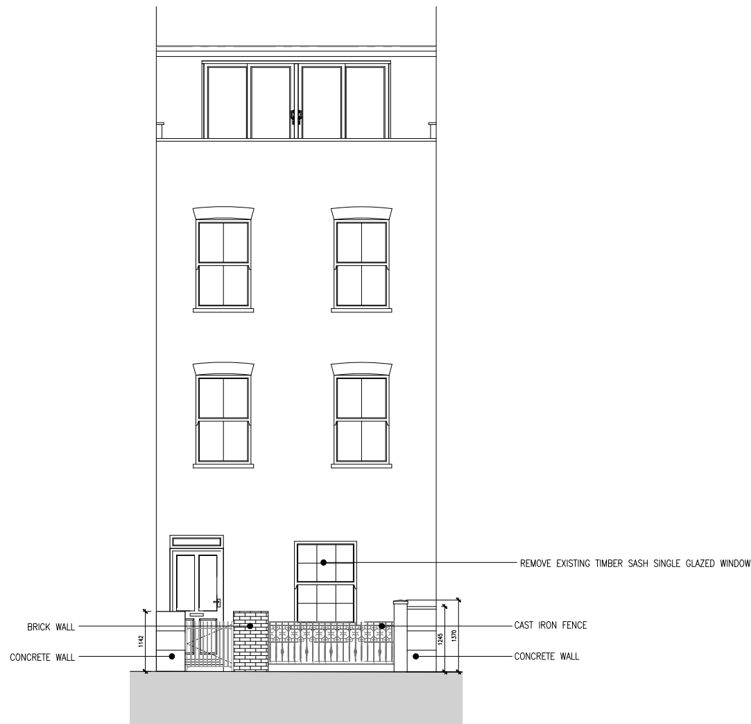
01 | EXISTING FRONT ELEVATION
