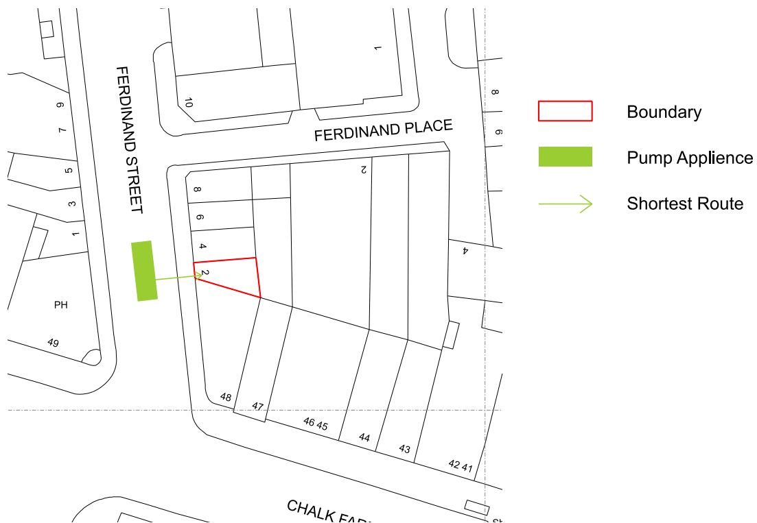
Site plan showing evacuation route and Fire Brigade access.
