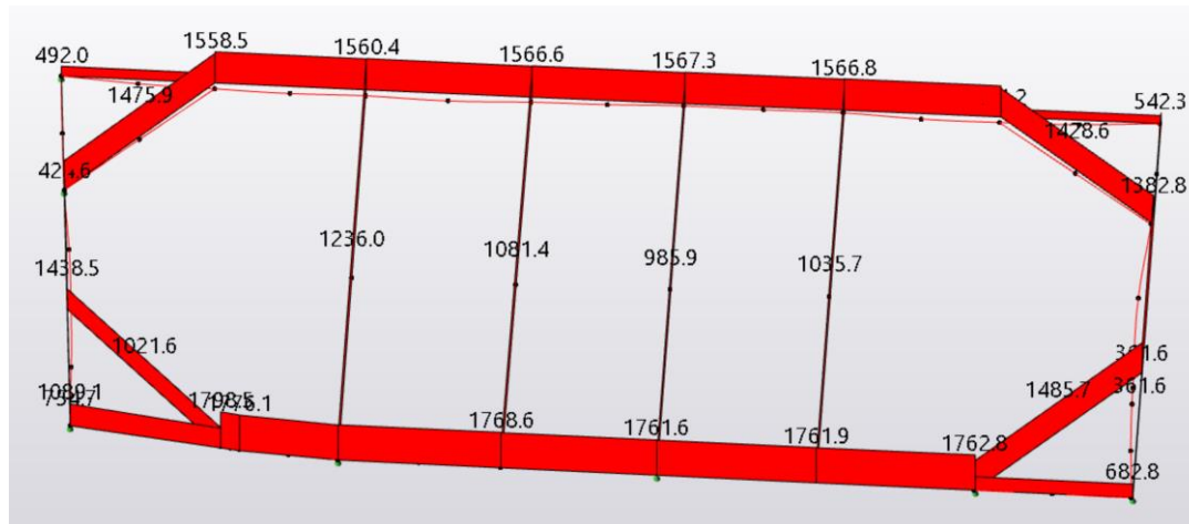
FIGURE 7 LEVEL 1 - PROP AXIAL LOAD - SLS
