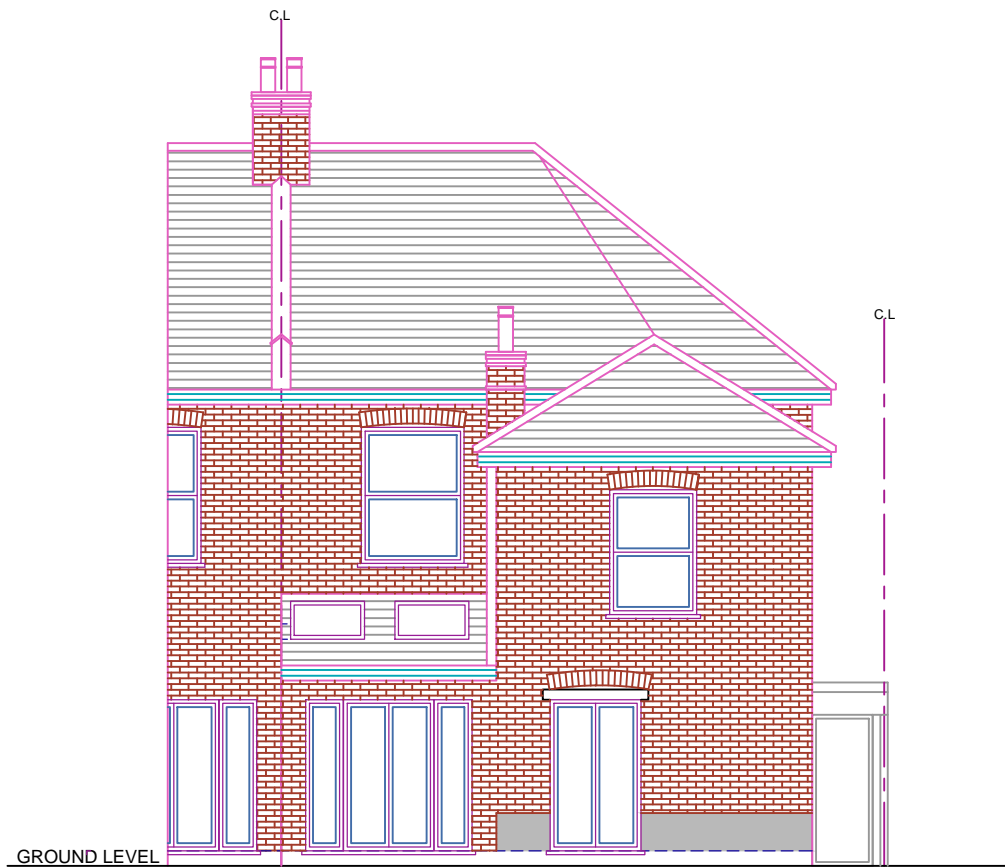
EXISTING REAR ELEVATION
