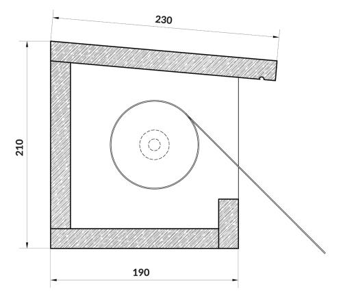
**Dimensions:**  $230 \text{mm} \times 210 \text{mm} (d \times h)$
