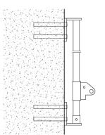
Fixing: Anchor bolt Size: M6 × 100mm Depth: 100mm (min)
