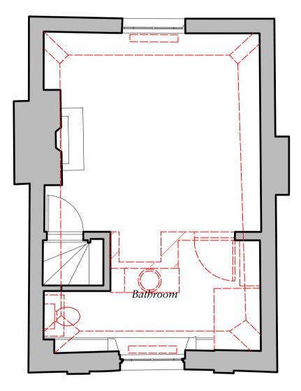
Proposed First Floor Removals Plan 1:50 All dimensions in millimetres. Where dimensions are not given, drawings must not be scaled and the matter referred back to Charlton Brown Architects.
