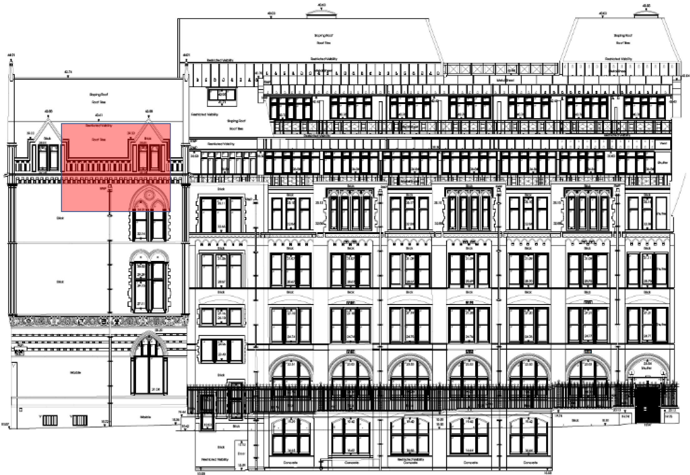
Leather Lane Lead Overflow Chute Location. Exact location demonstrated on below enlarged drawing.
