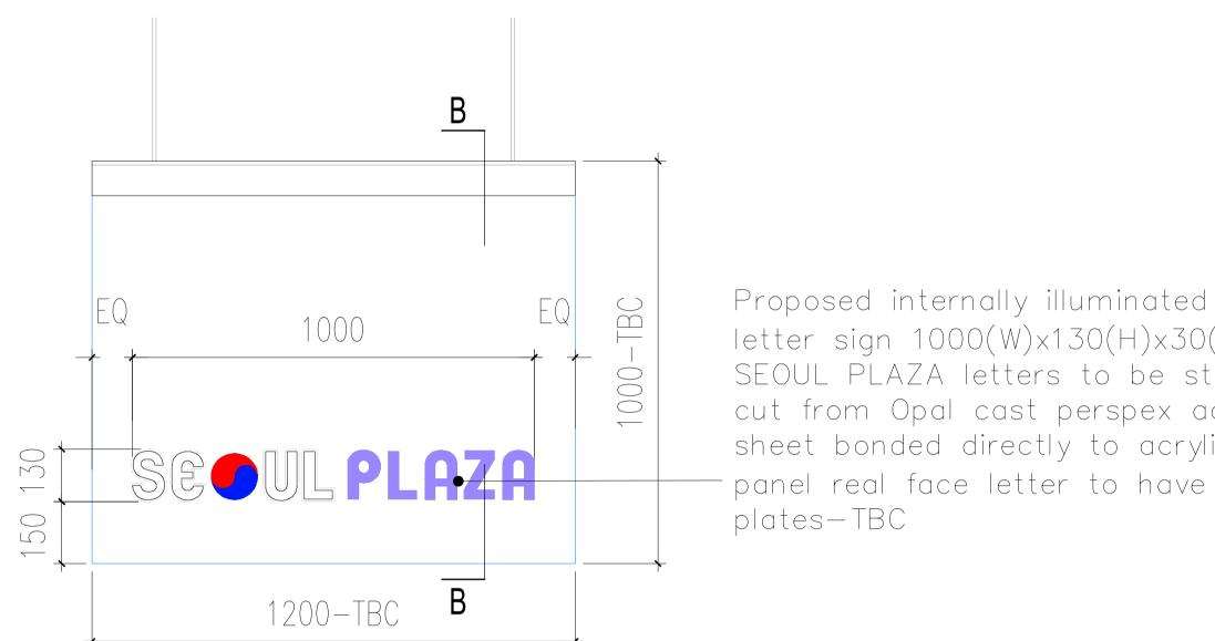
letter sign  $1000(W) \times 130(H) \times 30(D)$ mm, SEOUL PLAZA letters to be step cut from Opal cast perspex acrylic sheet bonded directly to acrylic panel real face letter to have s/s
