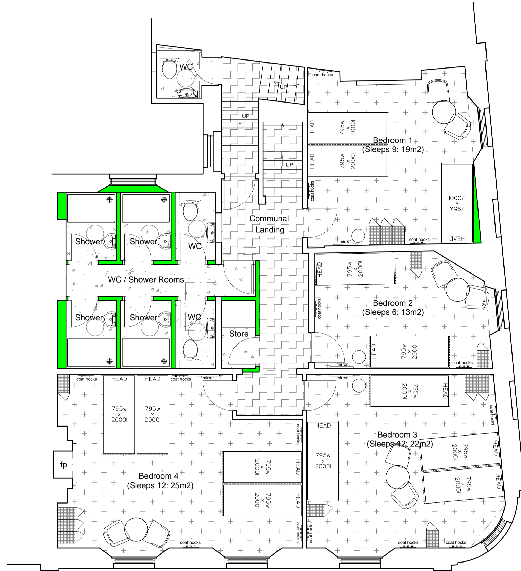
PROPOSED FIRST FLOOR PLAN SCALE 1:50 @ A1
