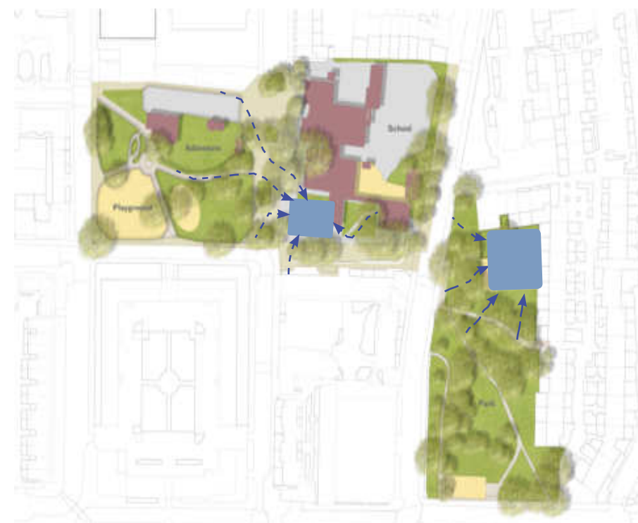
Fig. 5.6: Overland flowpaths in the vicinity of the existing site during extreme rainfall events
