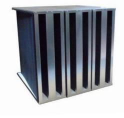
Our site safe carbon filters use panels of activated carbon to remove the malodourous gases within the commercial kitchen extract duct through the process of chemical adsorption. By installing adequate pre-filtration before our site safe filters, the carbon life span is greatly increased, allowing it to nullify malodours at optimum efficiency for much longer.
