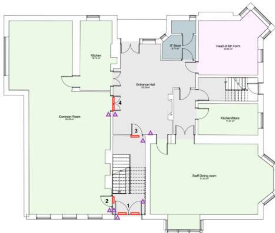
Figure 18 – Ground floor plan indicating the four doorways (numbered) requiring automation. Approximate location of the opening mechanism is indicated in red, and the proposed locations of command points to operate the doors are shown with purple triangles.
