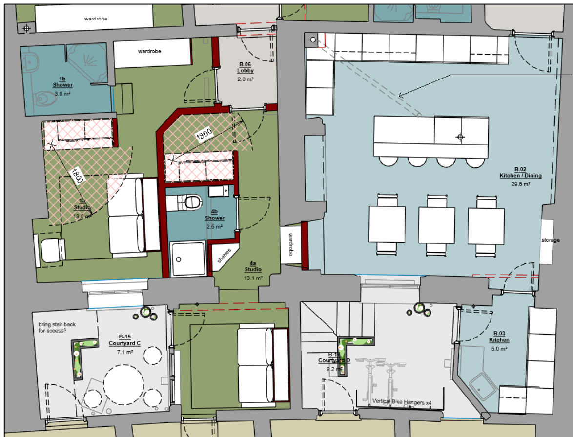
Figure 3.1 – Cooking facilities within Shared Living Units
