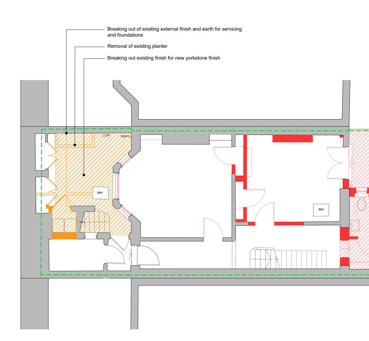
01 Proposed Demolition Plans - Lower Ground Floor D6199 SCALE: 1:50
