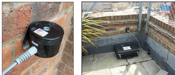
Example of Vibration Unit installation on wall
