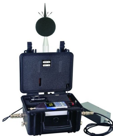
Example of Sound Meter within Weatherproof case and External Microphone
