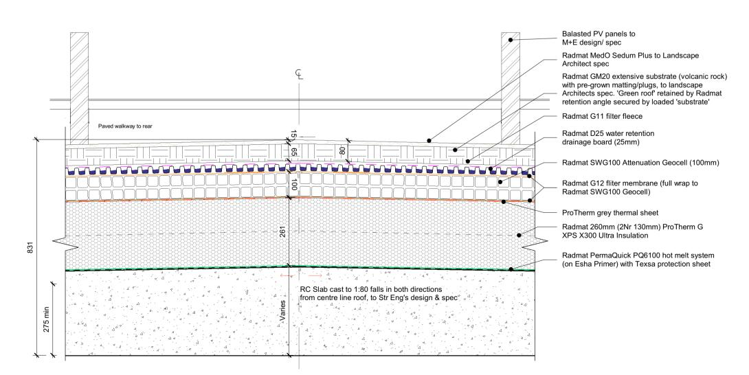
**5** Blue Green Roof Build-up - Block A with PV Panels
