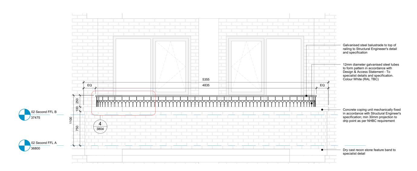
**Block A& C Type 1A Balustrade - Typical Elevation**1: 25
