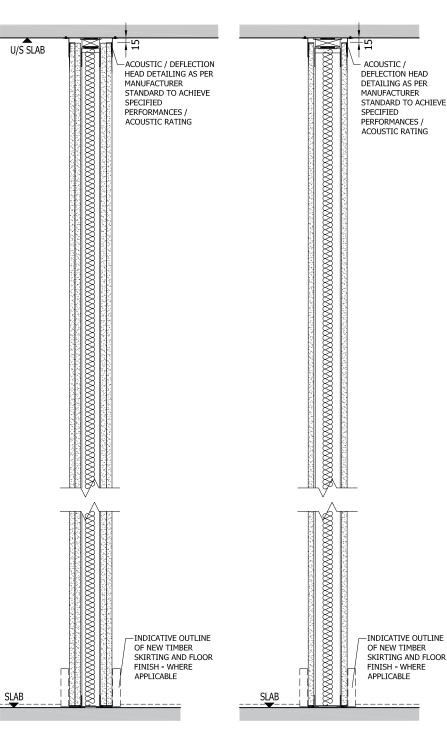
SOLID PARTITION TYPE P2: GYPWALL SINGLE FRAME SYSTEM REF: A206187 Fire Rating (integrity/insulation): 90/90 Acoustic Rating: 53 RwdB For detail; NBS spec K10/111
