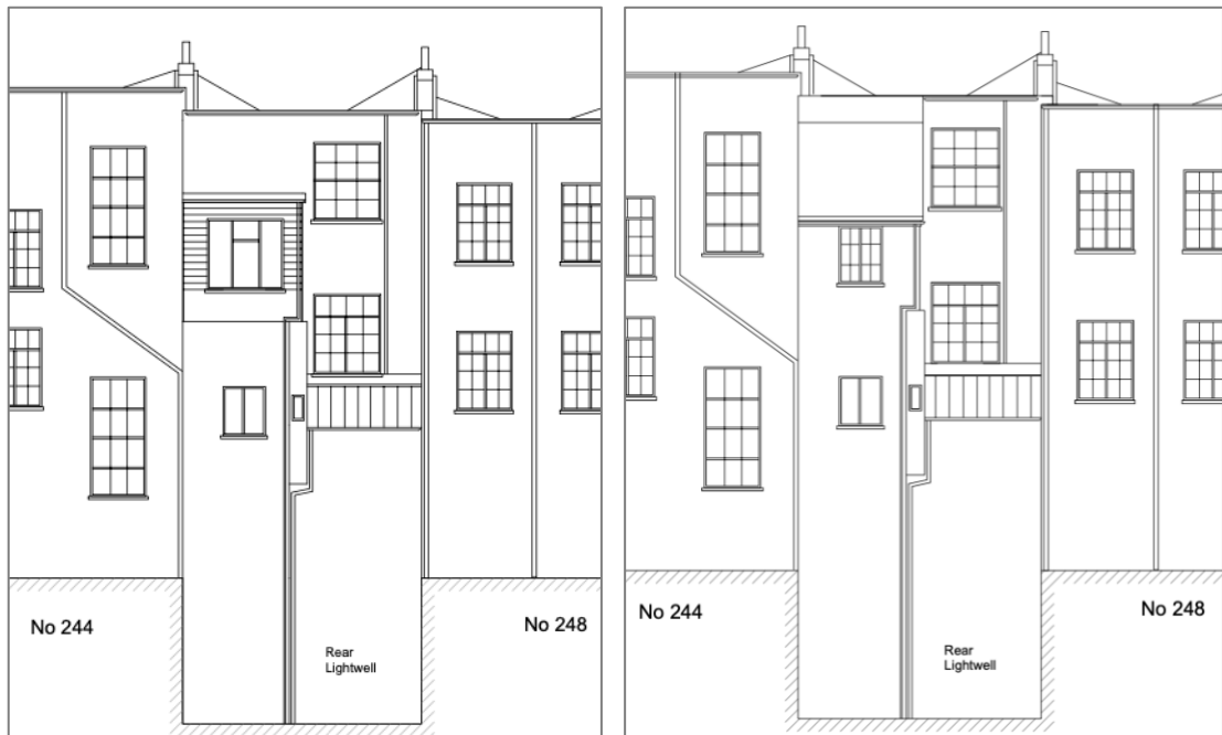
Figure 12: Existing and proposed rear elevation showing extension with smaller window, matching render and traditional sloping roof
