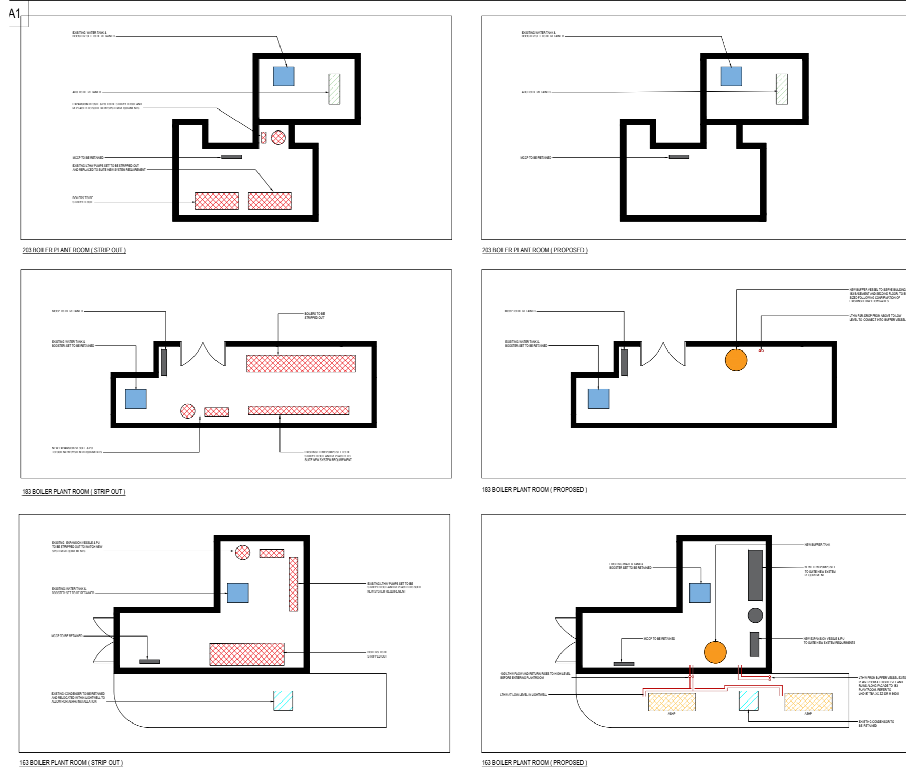
Figure 5.1 Proposed boiler plant refurbishments to 163, 183 and 203
