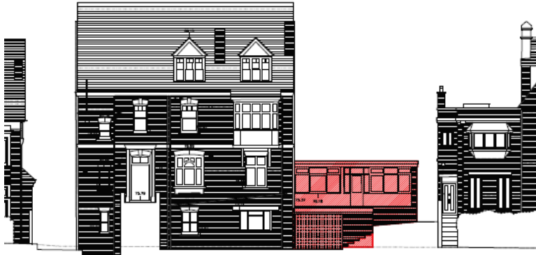
Image – front elevation of the existing building showing the proposed demolition in red
