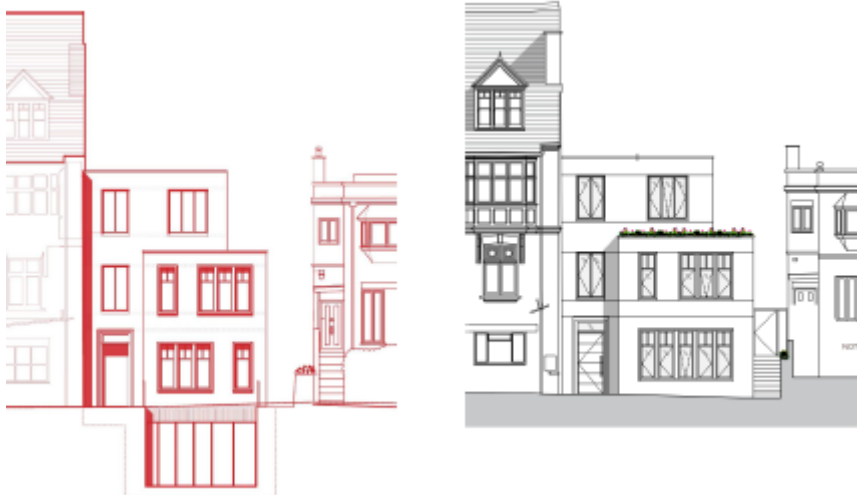
Front elevation - extant scheme out lined in red, proposed scheme in black
