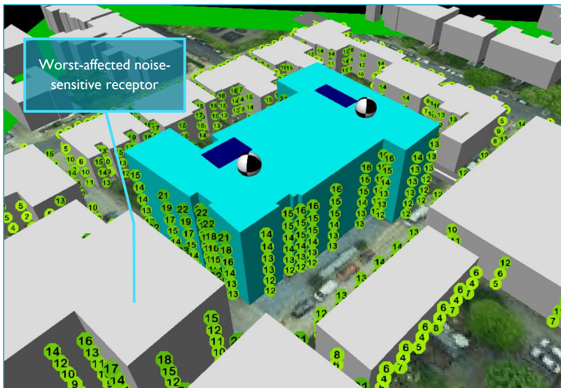
Figure 5 - Noise levels at the nearest noise-sensitive receptors (view from north)
