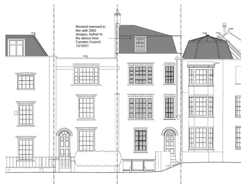
Right – The approved half hip-shaped mansard for no. 14 from 2021 by DMA (2021/4022/P)
