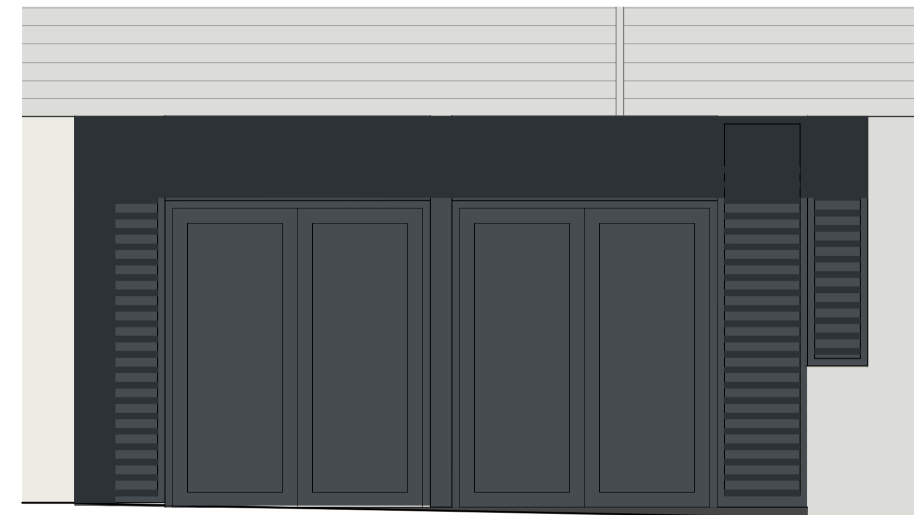
Electric Substation Elevation scale 1:50
