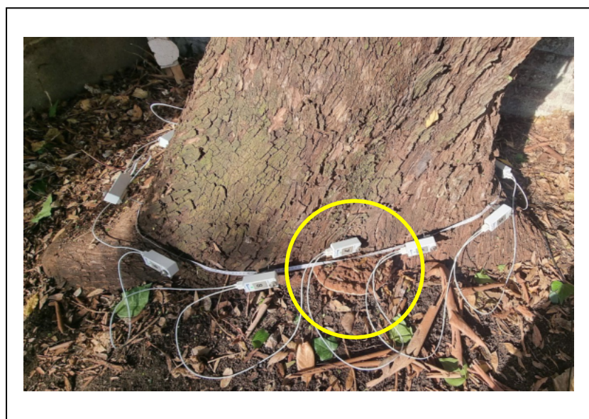
Figure 5. Close-up view of stem base and sensor positions, with Ganoderma sp. fungal fruit body circled at sensor position no.7
