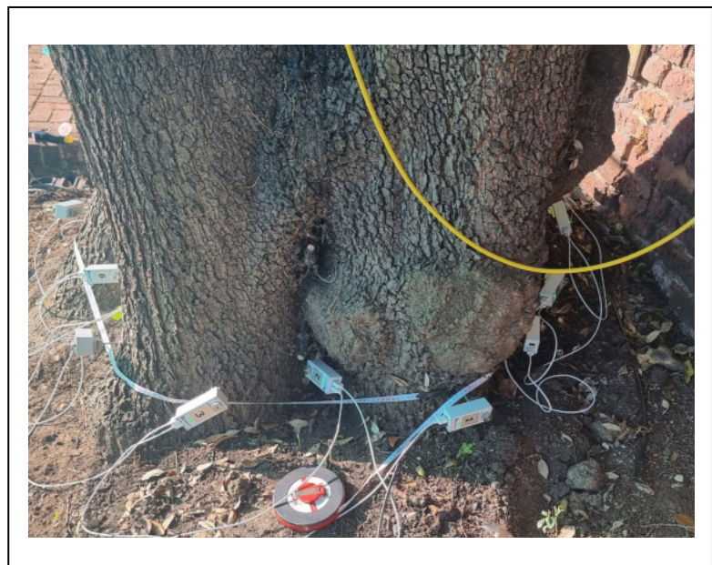
Figure 10. Close-up view of stem base with sensor positions, there is a small open basal cavity at position 10
