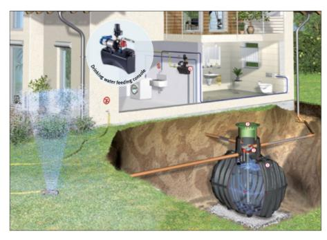
worth of water stored. The recommendation is 1,500 to 3,000 litres: Suitable for 1-4 people doing small amounts of garden irrigation. We have therefore specified a 2700 litre tank to be buried in the aarden alonaside the building. An automated pump
