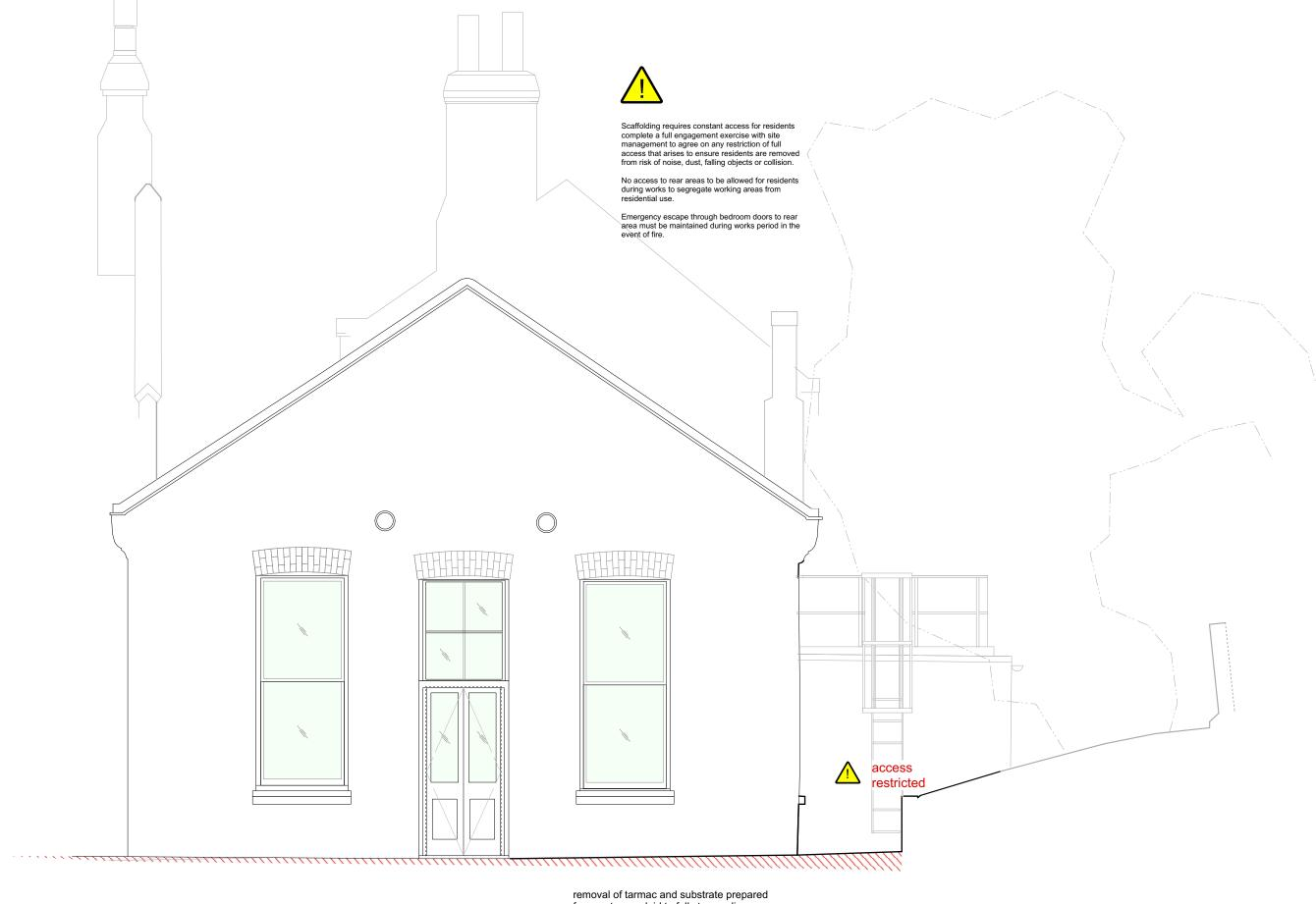
removal of tarmac and substrate prepared for new tarmac laid to falls to new linear drain connected to existing surface water system
