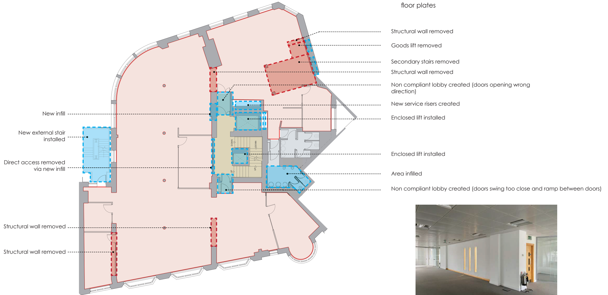
Typical floor plan Pre strip out works
