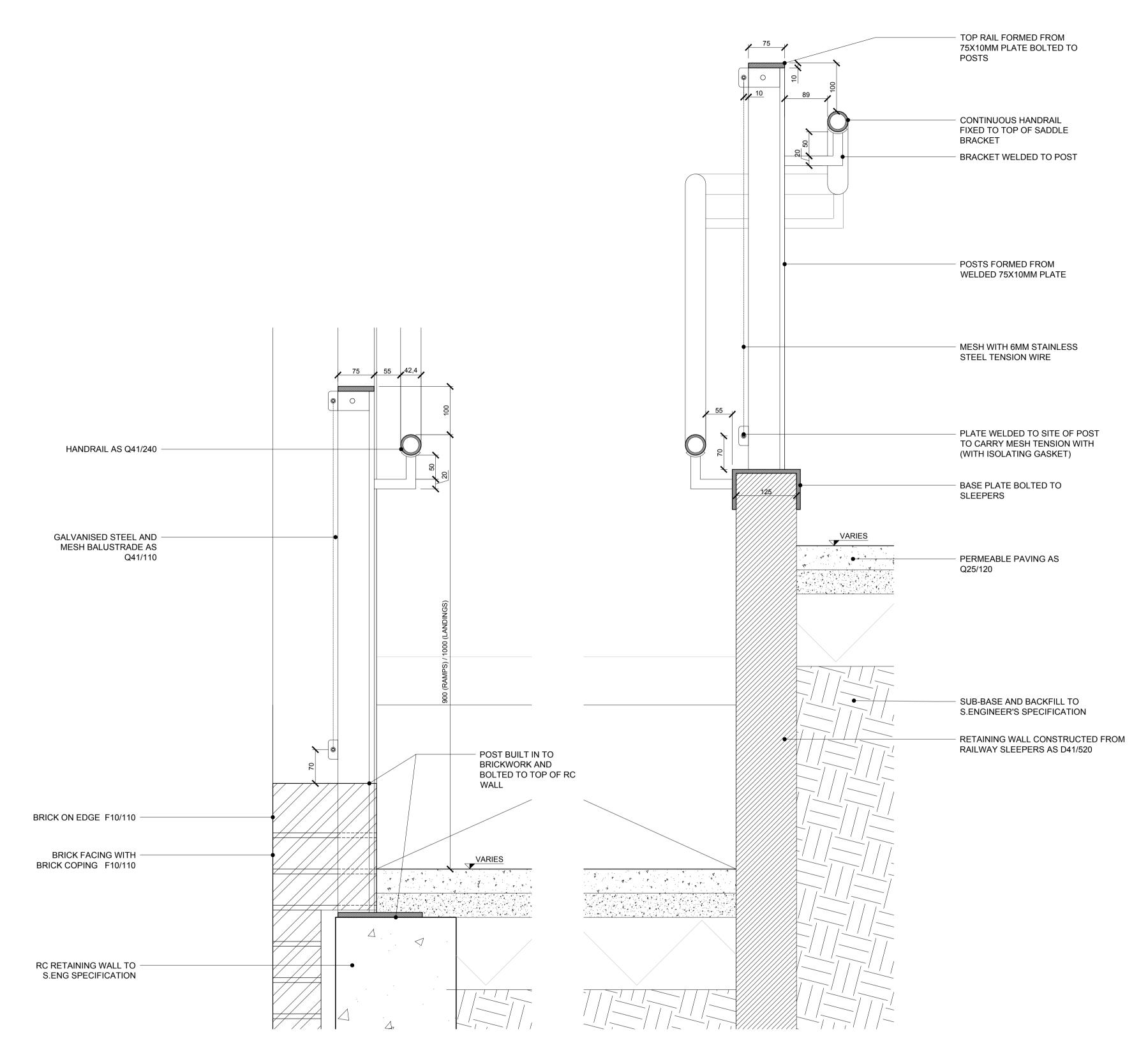
1. SECTION THROUGH HANDRAIL TO BRICK / RC RETAINING WALL
