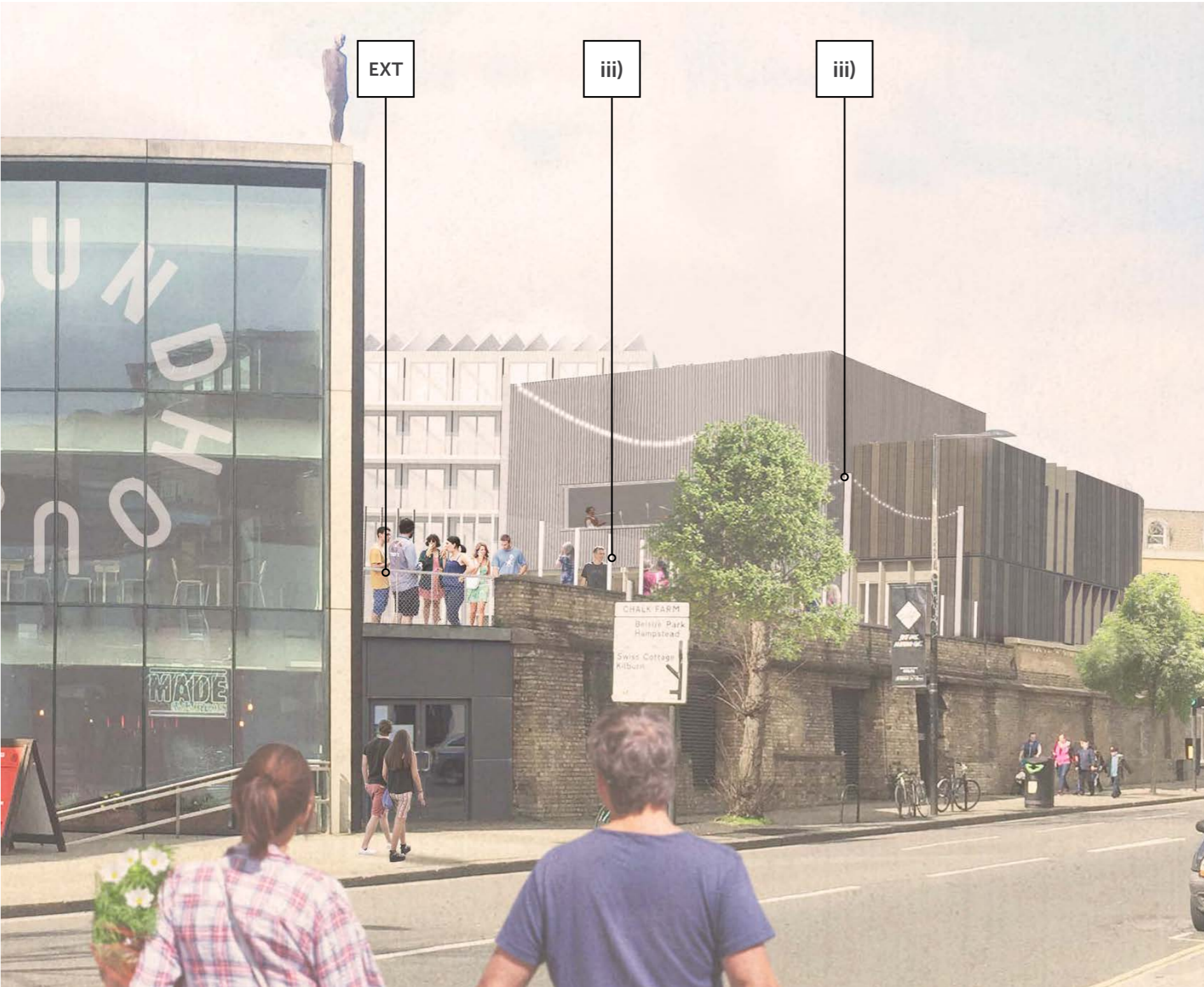
Image showing new balustrade / railings in relation to the existing buildings, new building and listed wall. 'EXT' = existing galvanised steel balustrade - see photo opposite
