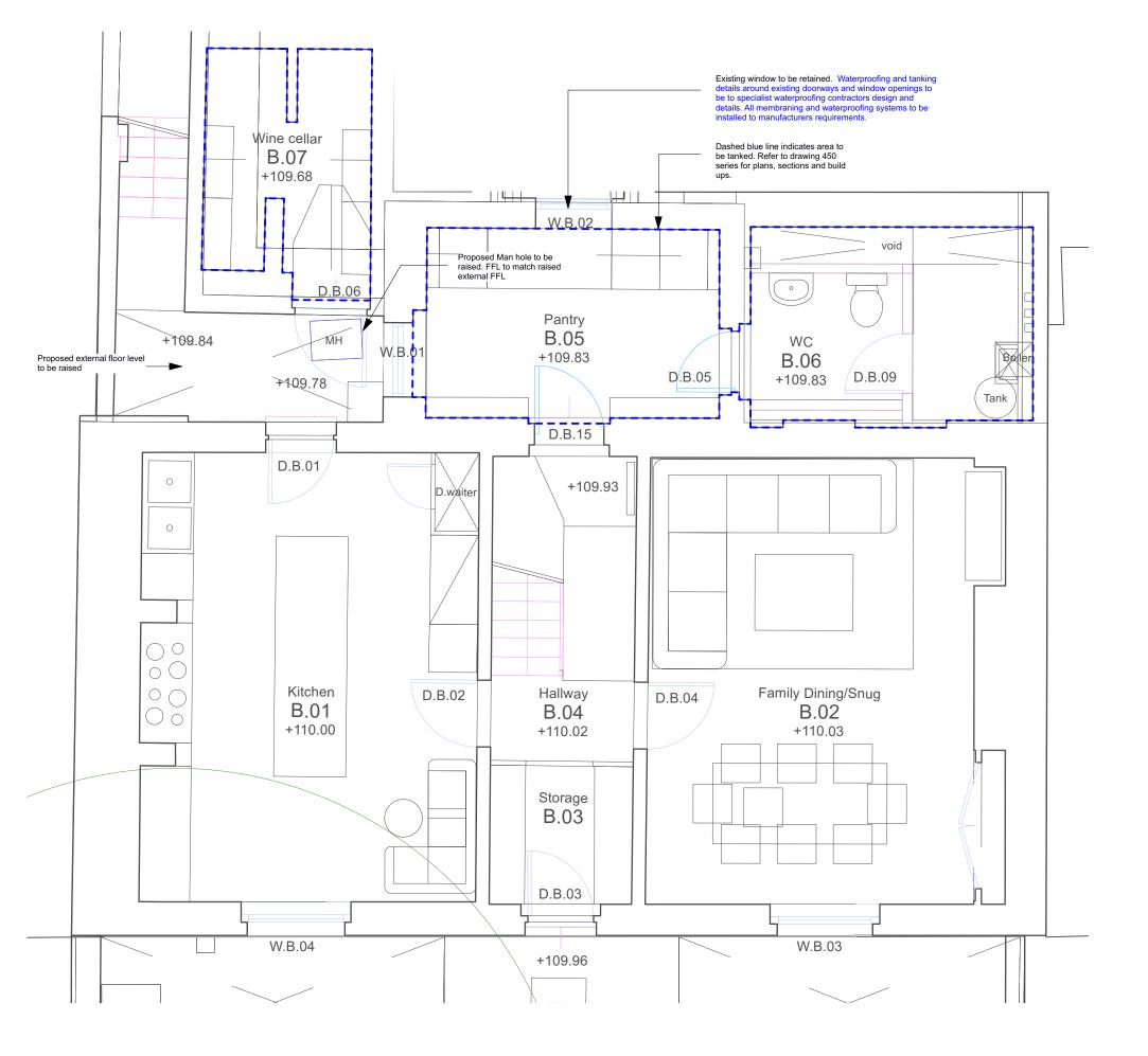
Proposed Basement Waterproofing Works Plan 1:50 @ A3
