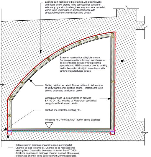
Proposed Basement GA Section [Through Utility] 1:25 @ A3
