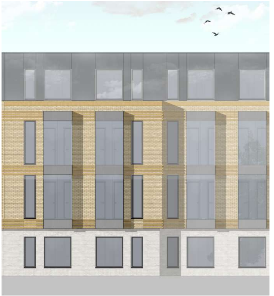
OPTION 4 Option 4 explores a different material for the top floor - back painted glass.
