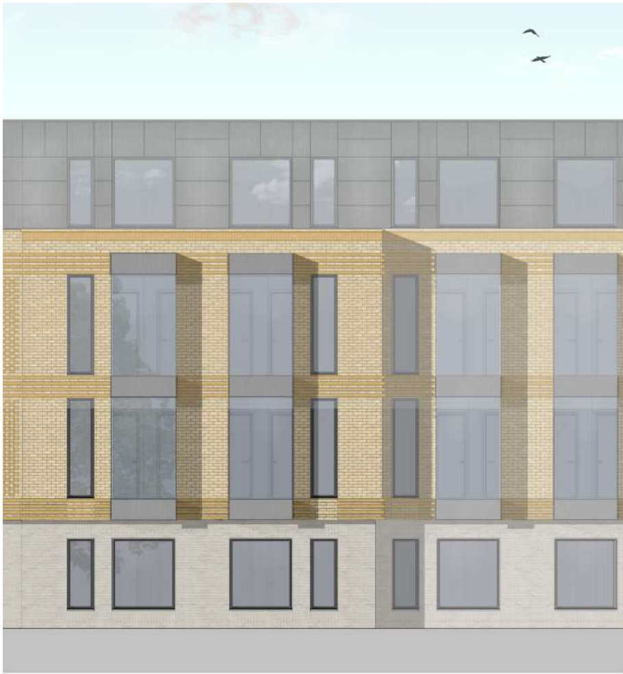
OPTION 3 Option 3 proposes identical brick selection for the main portion of the building. It introduces a slightly darker brick choice at Ground floor level and a Zinc clad top floor.
