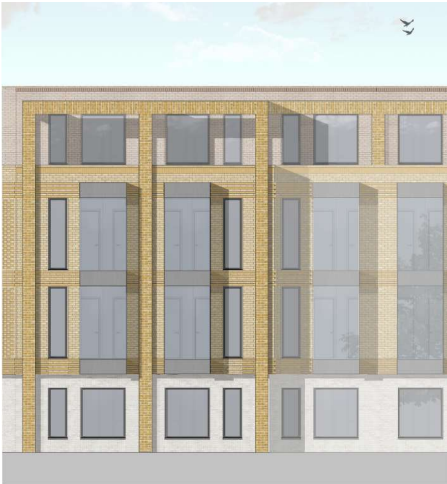
OPTION 2 Contemporary brick option with brick clad piers defining the bays of the building.
