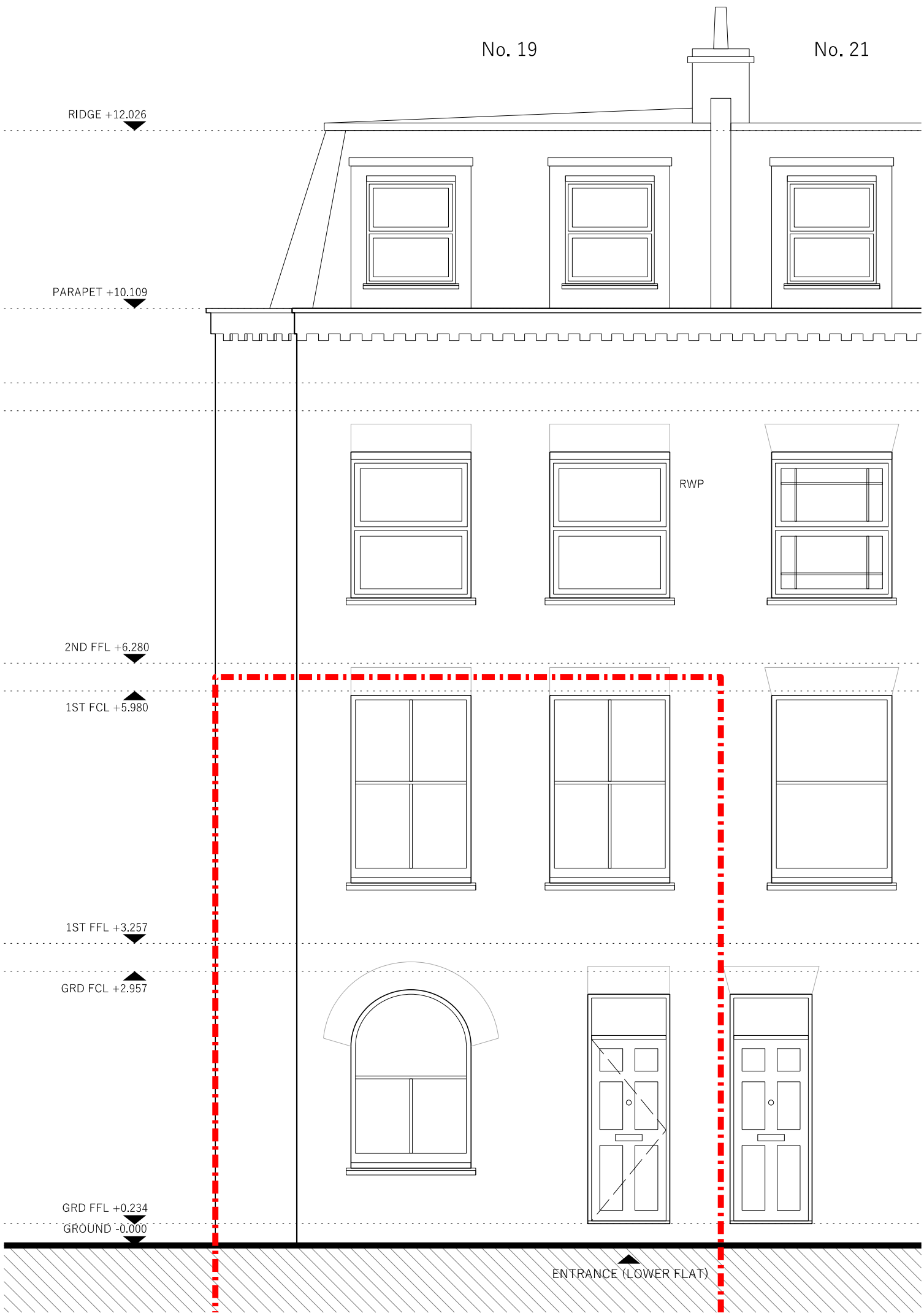
Existing Front Elevation
