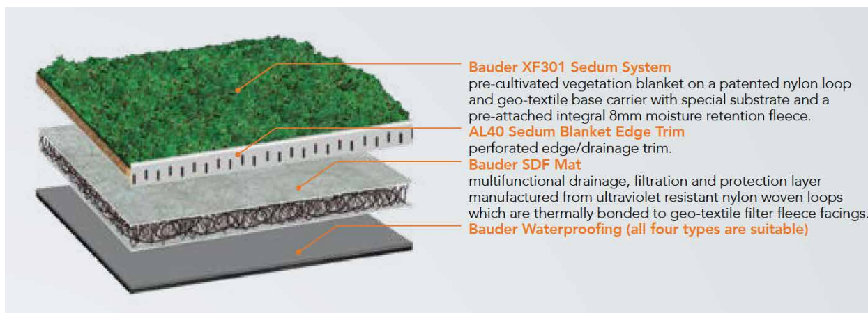
Example. Configuration of a lightweight sedum system (Bauder)
