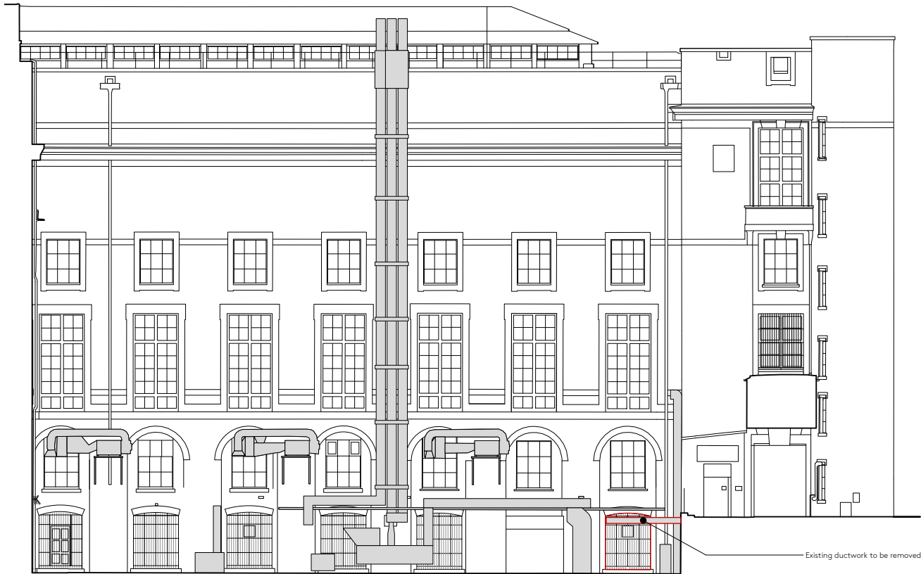
Southeast elevation of the KEB showing the window to be replaced, and the duct that is proposed to be removed.
